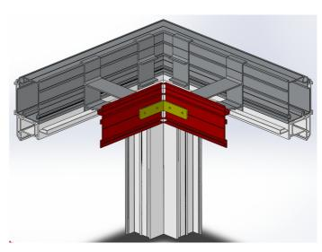
Offer up the UB200 under cladding and clip the Ring Beam Internal Trim into place.
