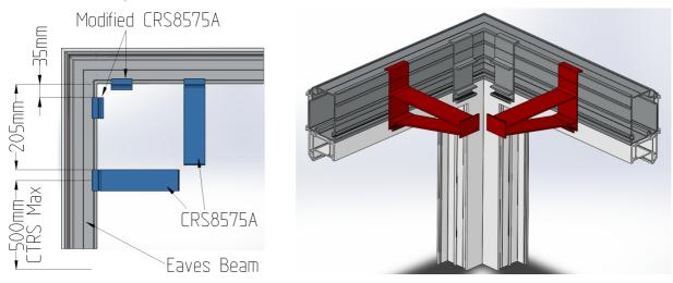
Once all brackets are in place screw them into position using 3.9x25 self drilling screws.
