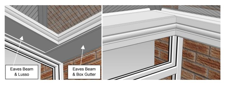
**OPTION 2** – Lusso and the Eaves Beam on the Box Gutter as shown below.
