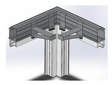
Locate the CB225 Capping board and screw into position.
