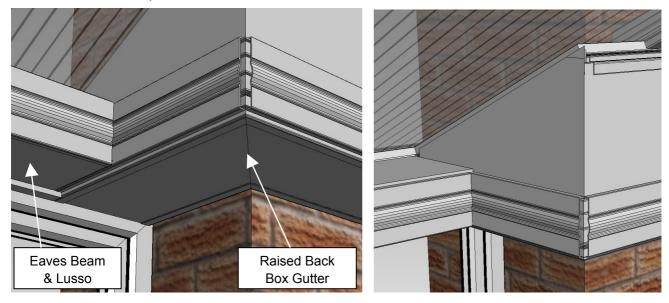
OPTION 2 - Lusso locates onto the Raised Back Box Gutter as shown below.
